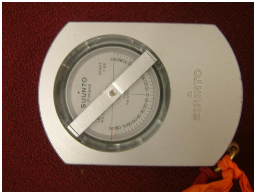
**Figure 14. Clinometer used to measure the height of the trees.**
