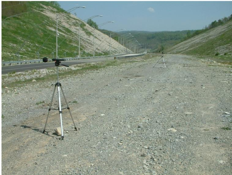
Figure 35. Sound level meter setup on the Smart Road.
