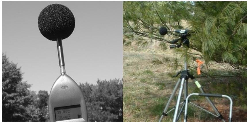
**Figure 6. Use of windscreen on an SLM.**
