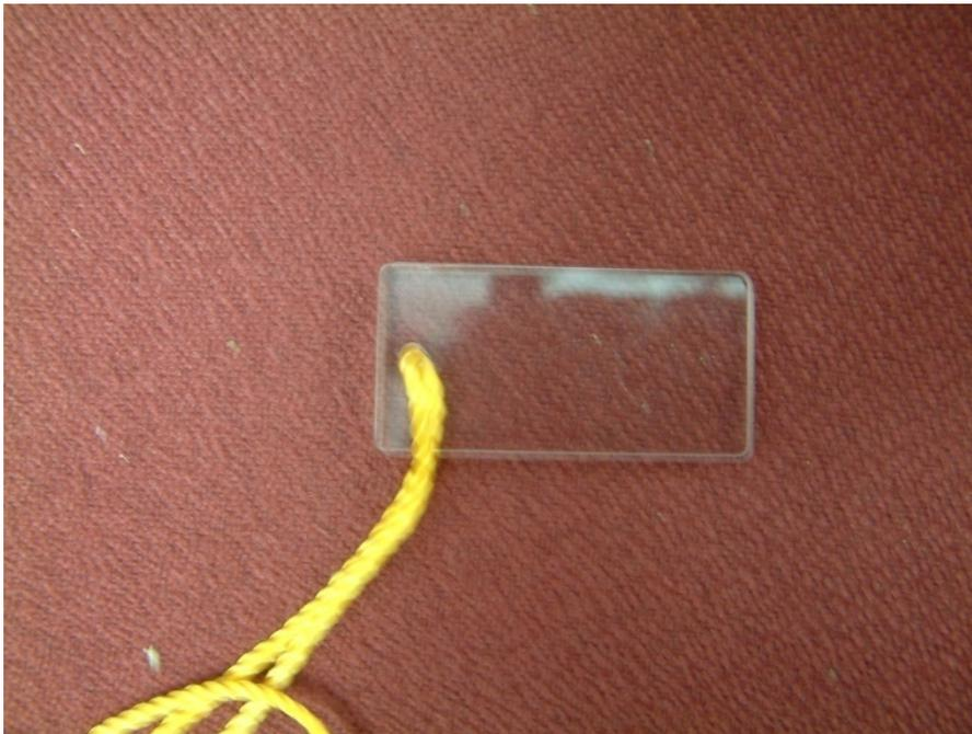
**Figure 15. The BAF 10 prism used to measure basal area of each plot (a measure of tree density).**
