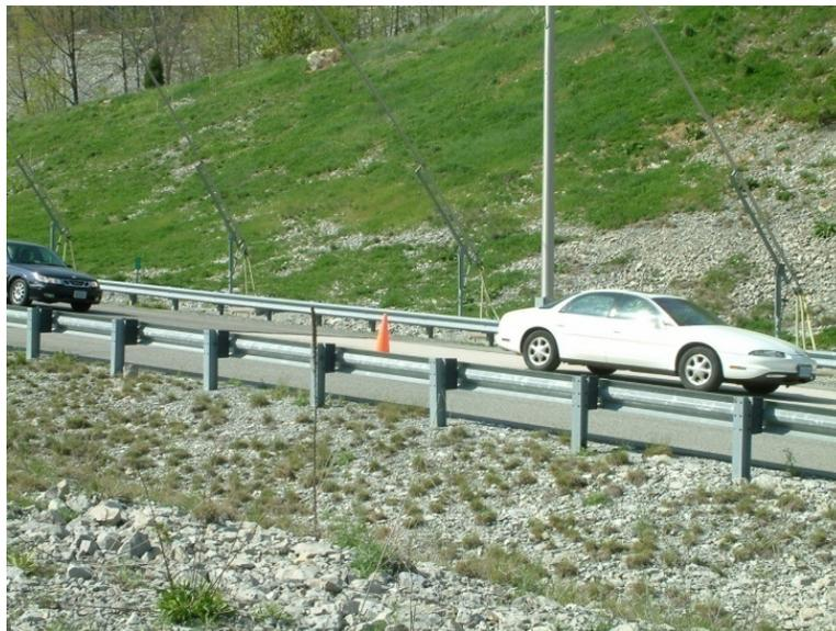
**Figure 38. Dual light vehicles going downhill. Measurement started when the front of the first vehicle crossed the entrance cone and ended when the rear end of the second vehicle crossed the exit cone.**
