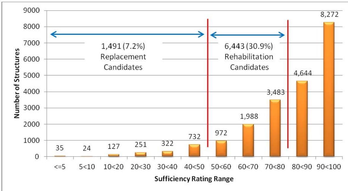
**Figure 17 Bridge and Culvert Sufficiency Rating Ranges**
