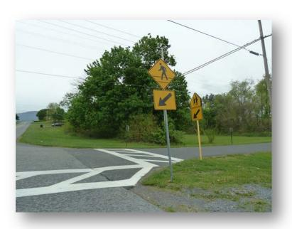
Intersection of Second Street and Luray Avenue – on Luray Avenue looking east. Ladder-style crosswalks and pedestrian signage help make motorists aware of pedestrians crossing the street. However, these signs are inconsistent with each other and could be replaced with the neon yellowgreen signs for higher visibility. Also, the lack of sidewalks along Luray Avenue can make pedestrians less comfortable when walking along the street.
