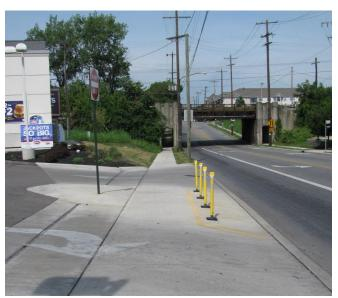
Access management in Columbus, Ohio: Flexible bollards and pavement markings direct motorists to both the entrance and exit along the wide driveway.
