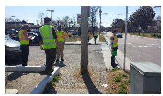
Figure 20: At Sewell's Point Road and Strand Street, the crosswalk on the north side lacks curb ramps while the crosswalk on the south side connects to a driveway
