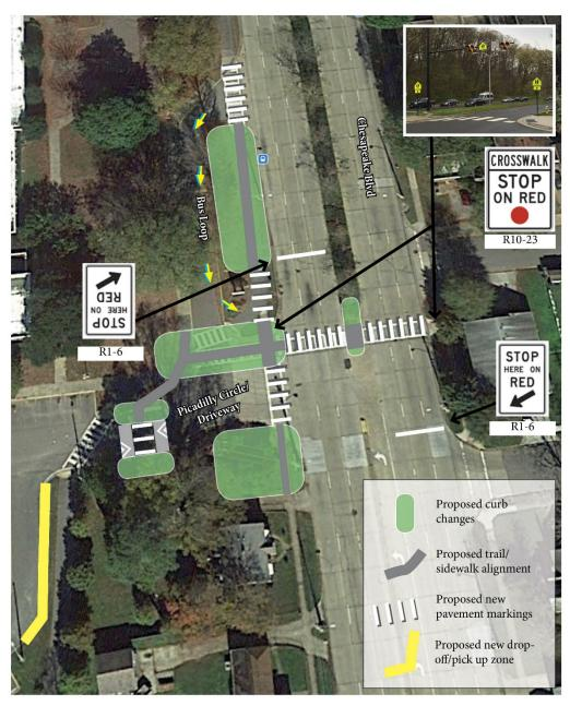
Figure 8: Concept for Recommended Improvements on Campus and at the Picadilly Circle/Chesapeake Road intersection.
