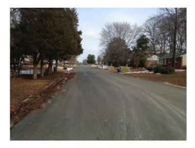
**Figure 2.Perlock Road (facing east).** Perlock Road is the second key access route to Bellwood Elementary School from the Quail Oaks neighborhood and Jefferson Davis Highway. Both Perlock Road and Galena Avenue are relatively wide, unstriped (32-33 feet) and do not have any STOP controls between Jefferson Davis Highway and the school, which may encourage speeding.
