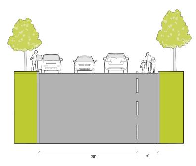
Figure 10. Proposed short-term cross section
