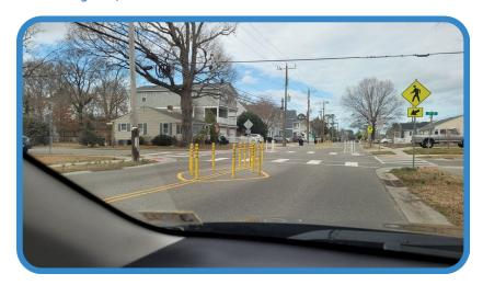
Figure 18. Example of flex-post median in Virginia Beach, VA
