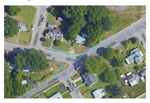
Figure 21. Sketch of intersection reconstruction, where blue lines indicate the new curb line
