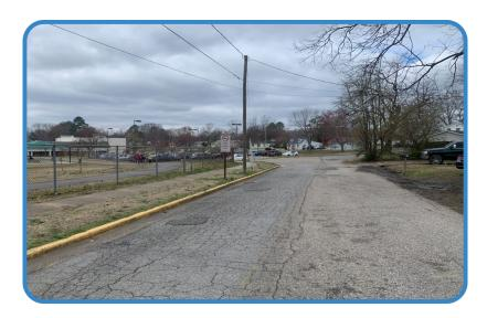
Figure 14. The pavement along the school driveway is in poor condition.
