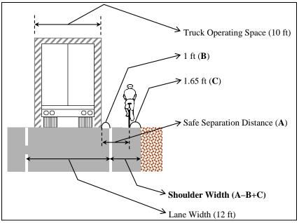
Figure C-2. Shoulder width calculation.
