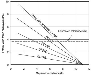
Figure 2. Aerodynamic forces caused by heavy vehicles passing bicycles (Figure 4-8, FHWA, 1977)
