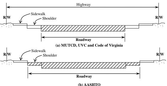
(b) AASHTO Note: R/W represents right of way. Figure 1. Difference in definitions of highway and roadway.
