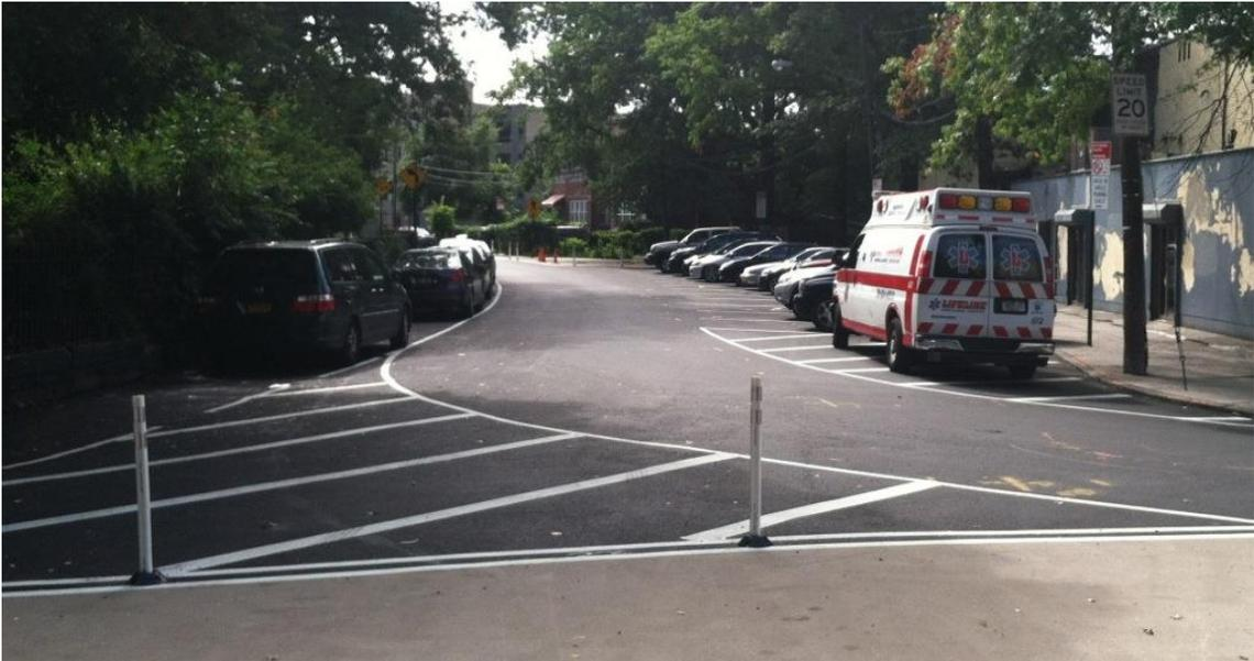
**Figure 2.3 - Narrow travelway by re-striping to add parallel parking lanes**
