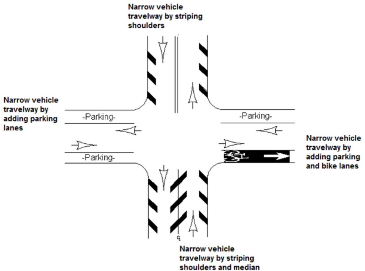
**Figure 2.2 –Narrow travelway by re-striping pavement**
