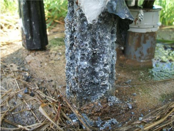
Corrosion with 1/8" deep pitting on breakaway couplers
