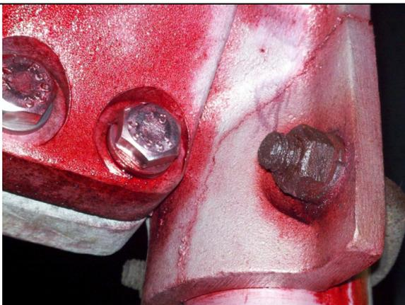
Crack in orbital bracket of 2nd signal from right pole
