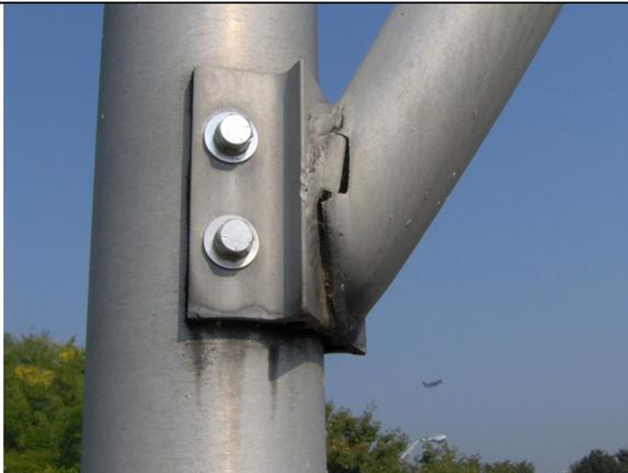
Fracture in weld of lower arm tube to luminaire pole connection
