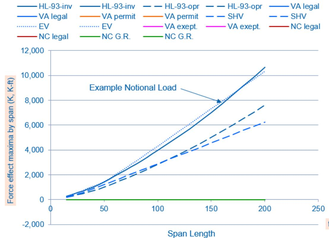
**Actual vehicle force effects should be less than the notional load**
