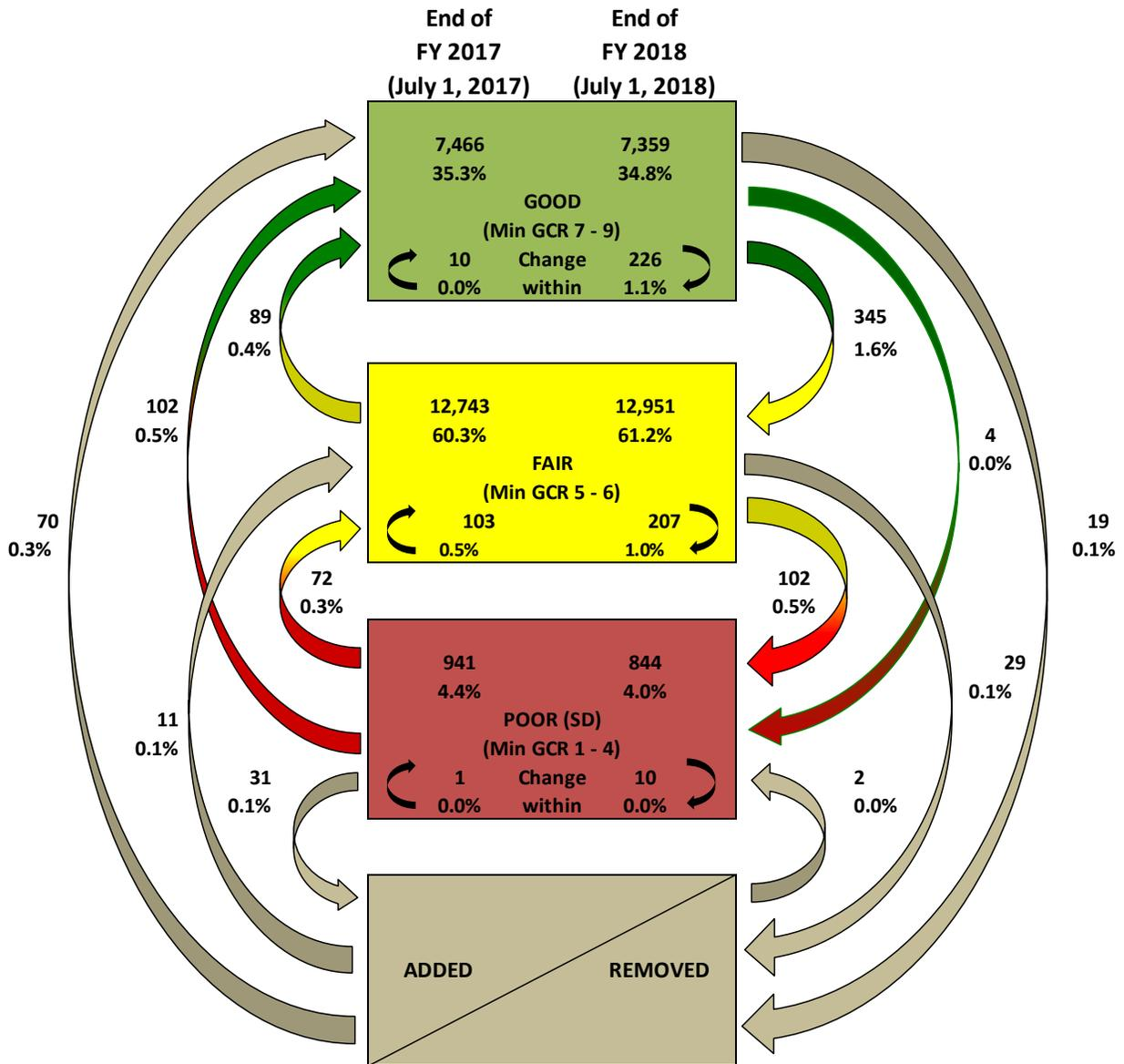
Figure 3-2- Annual Transitions of Good/Fair/Poor or Poor (SD) from End of FY 2017 to End of FY 2018
