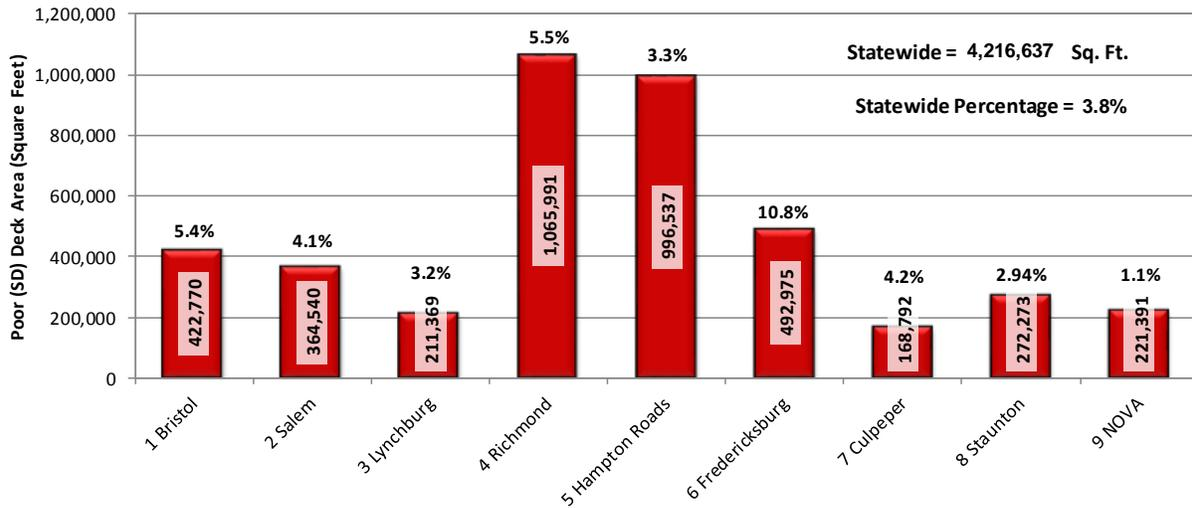
Figure 3-17- Deck Area of Poor (SD) Structures by District
