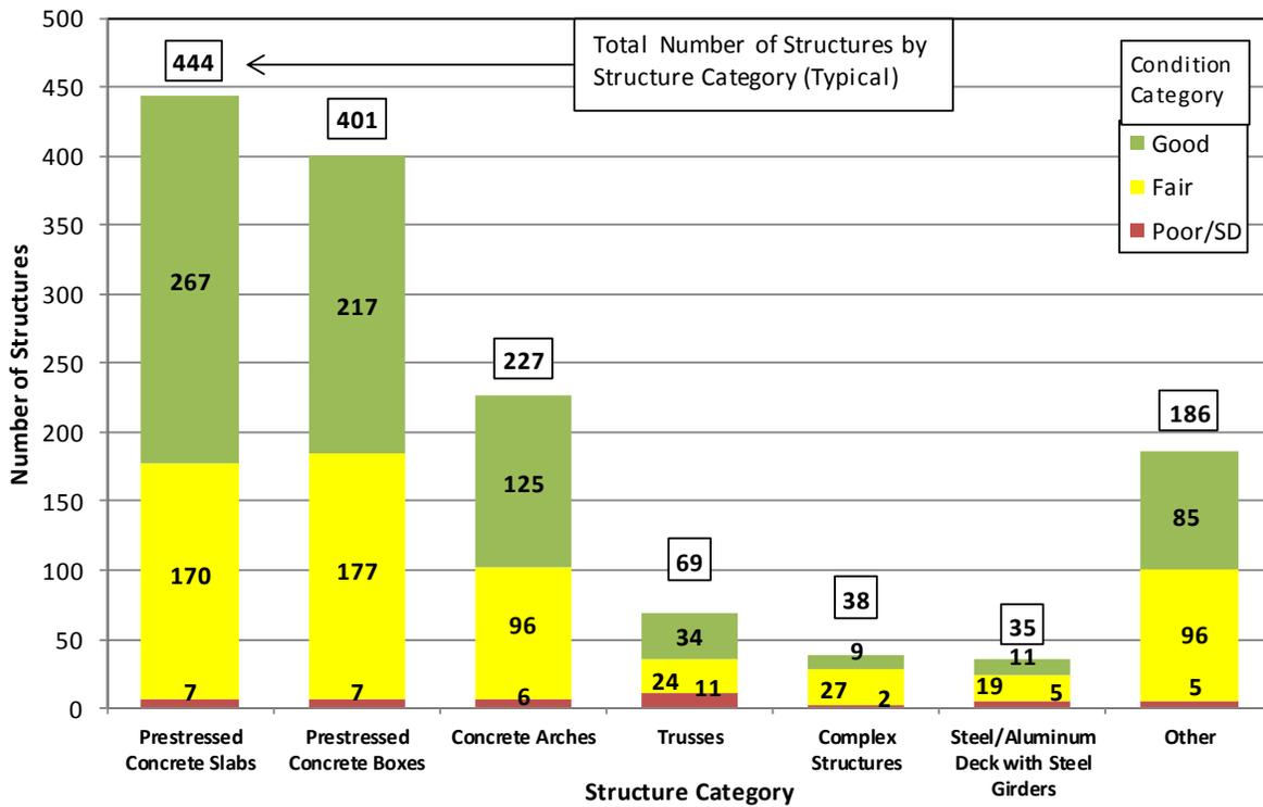
Figure 2-5- Count and Condition Data for Less Common Structure Categories (All Structures)
