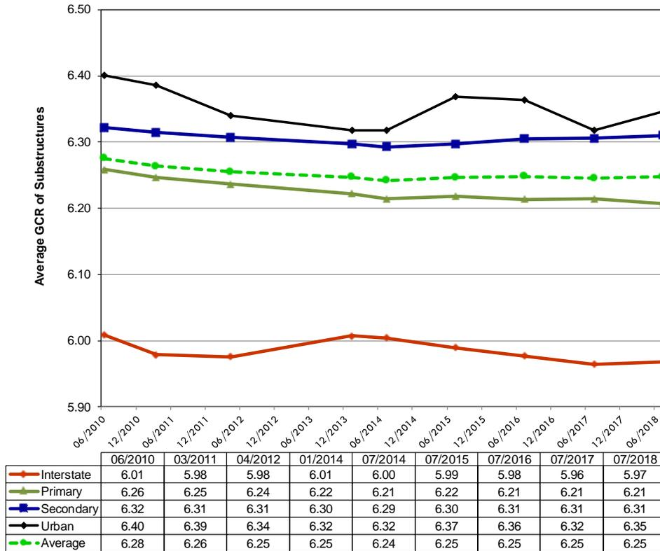
Figure C-4- Substructures: Trends in Average General Condition Ratings by Highway System
