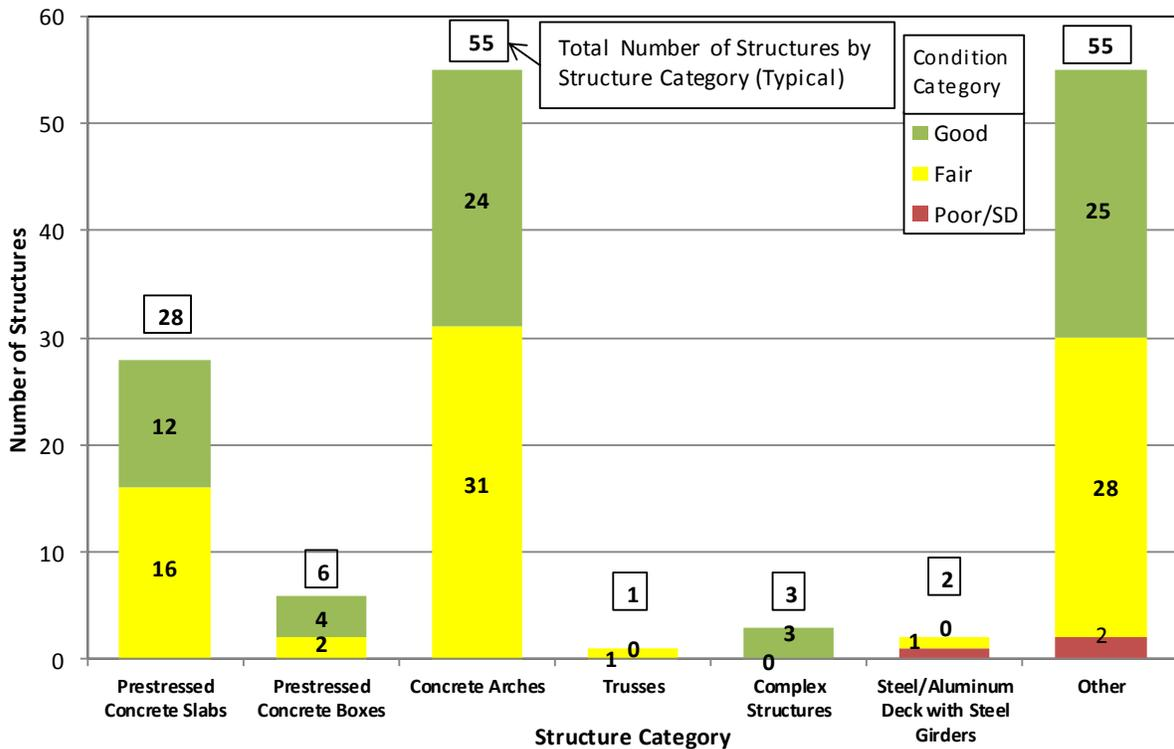
Figure 2-9- Count and Condition Data for Less Common Structure Categories (Non-NBI Structures)
