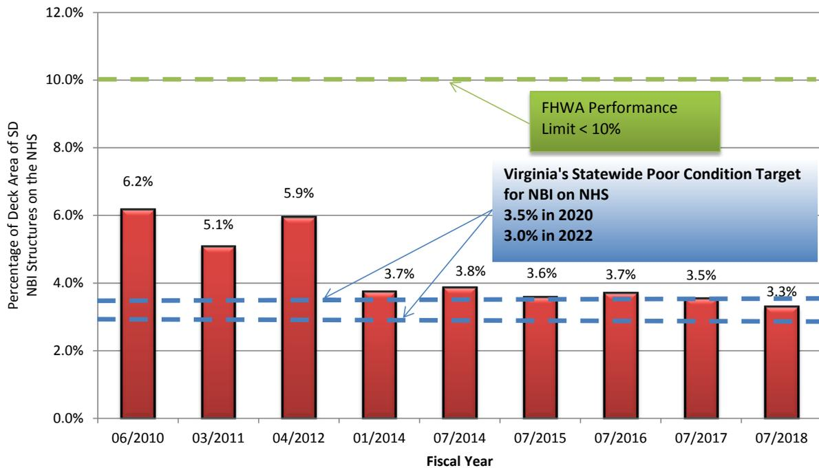
**Figure 3-3- Percentage of Deck Area of Poor (SD) NBI Structures on the NHS by Year**
