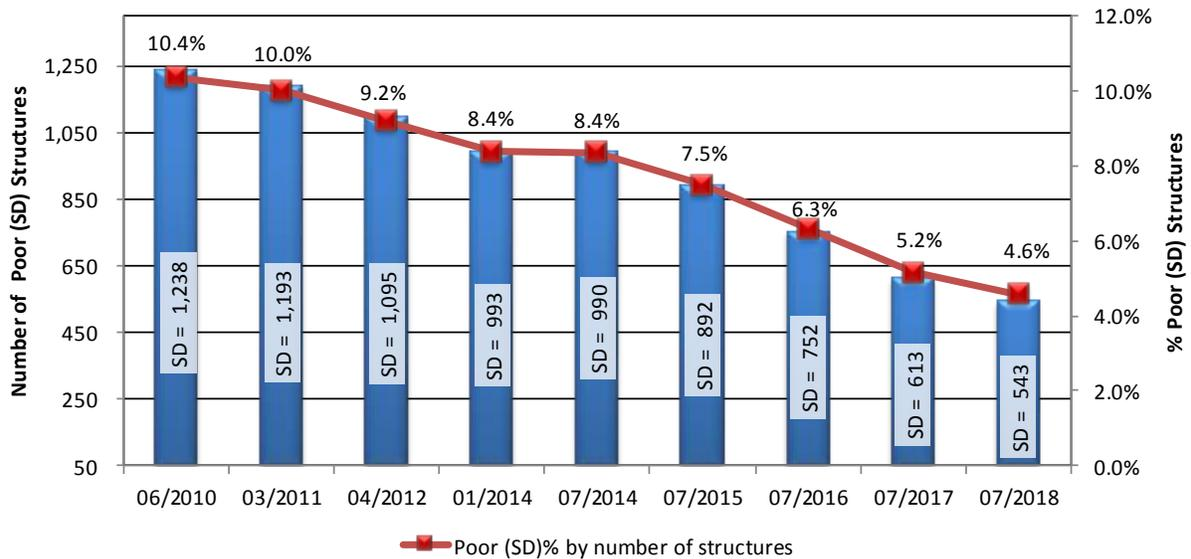
Figure 3-23- Percentage of Poor (SD) Structures - Recent Trends for Secondary System
