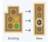
Example of a 5 to 4-head traffic signal conversion using a flashing yellow arrow
