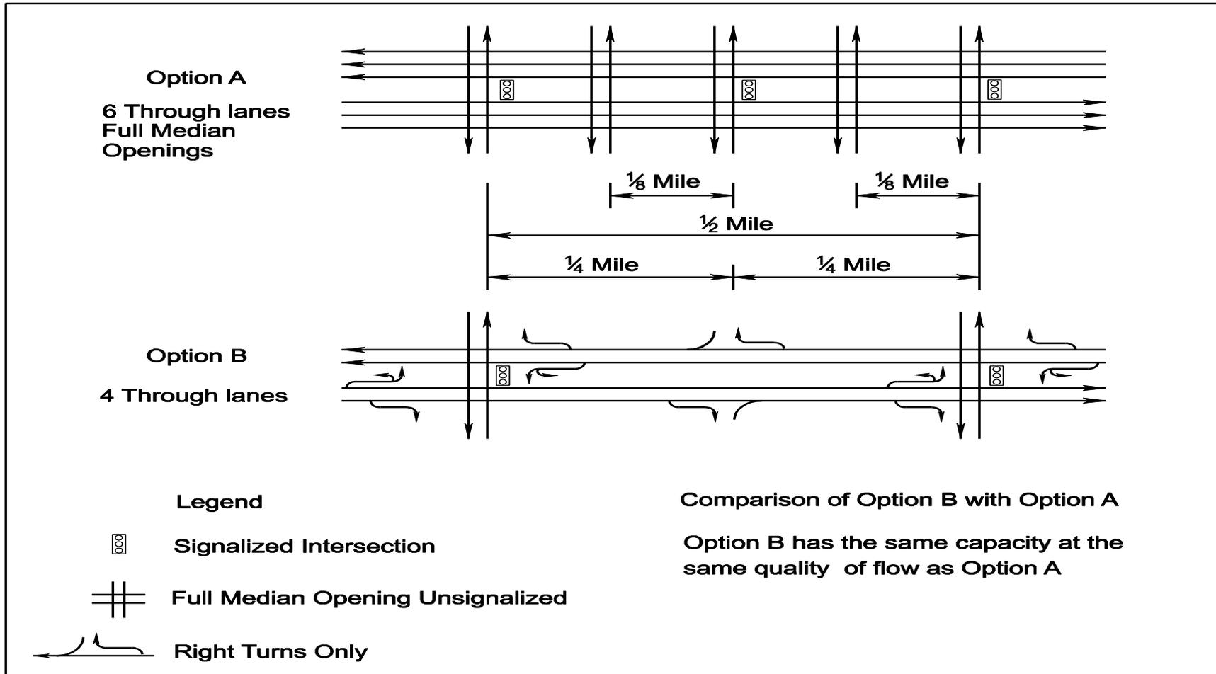
**FIGURE 2-8 ILLUSTRATION OF ENTRANCE AND INTERSECTION SPACING**
