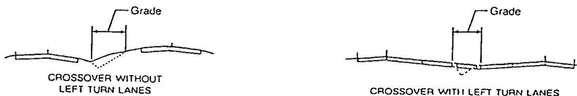
In preparing plans for field inspection, the gradient at each median crossover is to be plotted graphically.
