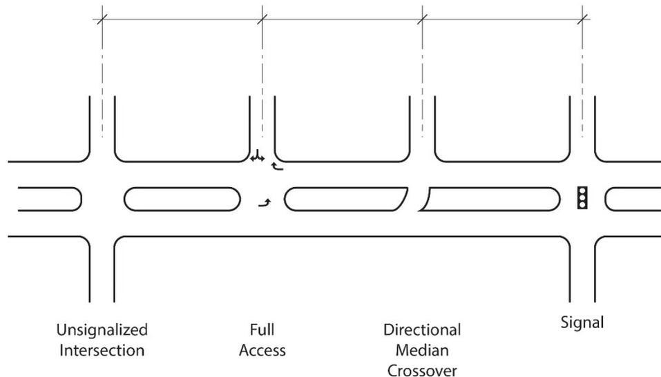
Spacing can be less than unsignalized intersection and full median crossover spacing. Full accesses on a four-lane roadway have only 11 potential conflict (collision) points and directional crossovers on a four-lane roadway only have six. However, studies have demonstrated that the majority of access-related vehicular crashes involve multiple left
