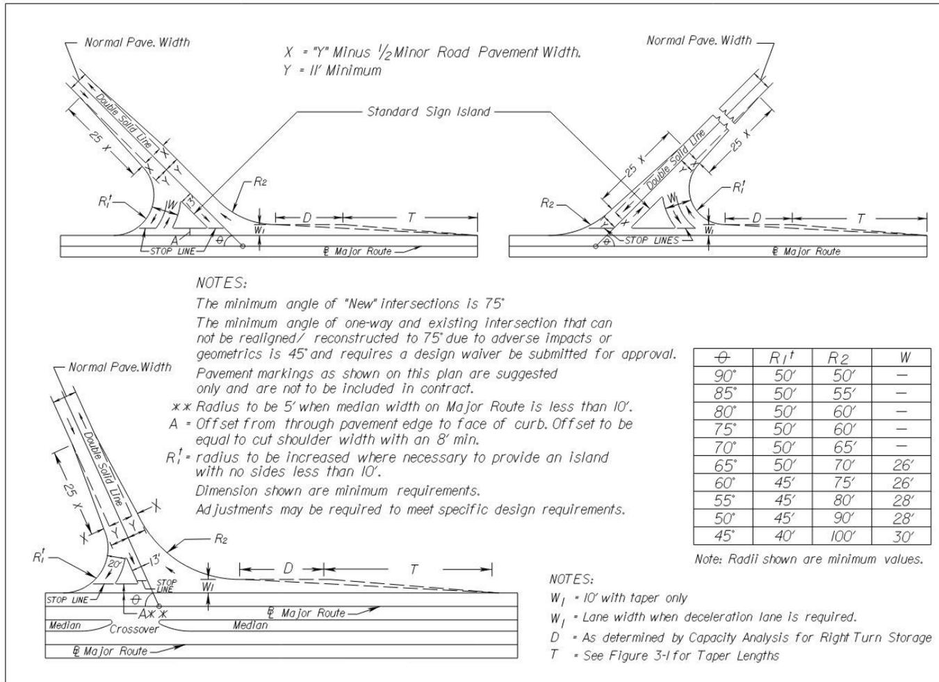
**FIGURE 2-12 INTERSECTION DESIGN FOR RURAL APPLICATIONS WITH OR WITHOUT STANDARD SI-2 OR SI-3 SIGN ISLAND DESIGN\***
