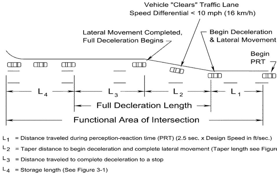
**FIGURE 4-3 ELEMENTS OF THE FUNCTIONAL AREA OF INTERSECTION**
