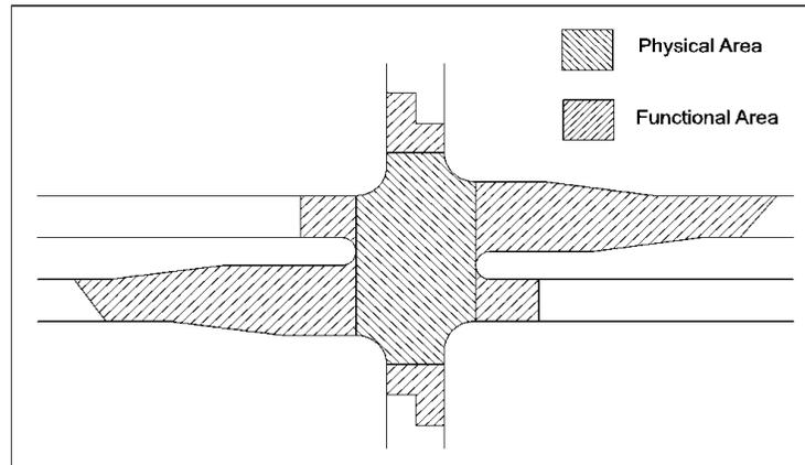
**FIGURE 4-2A PHYSICAL AND FUNCTIONAL AREAS OF INTERSECTION**
