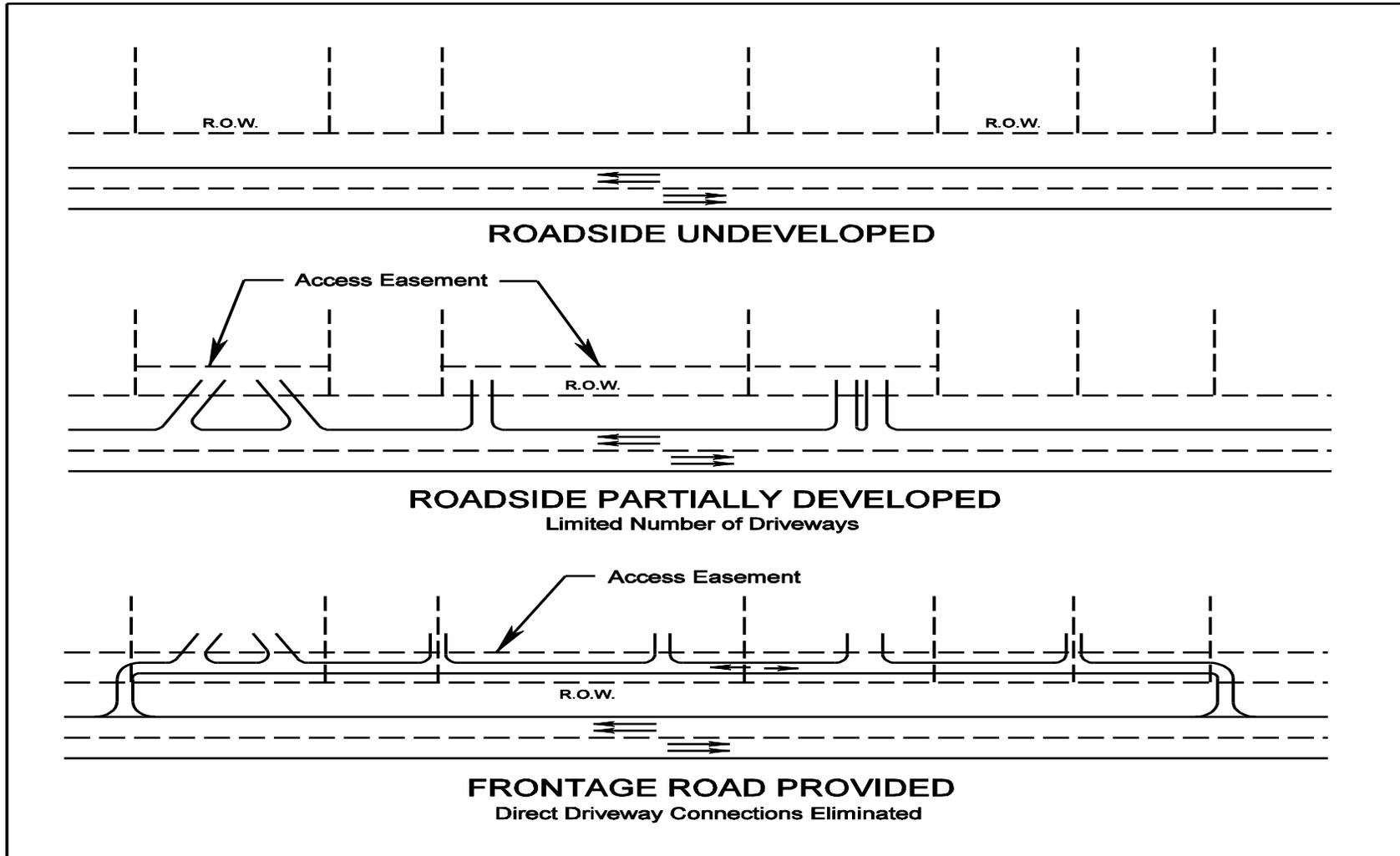
**FIGURE 2-7 ACCESS DEVELOPMENT SCENARIO ALONG A STATE HIGHWAY**
