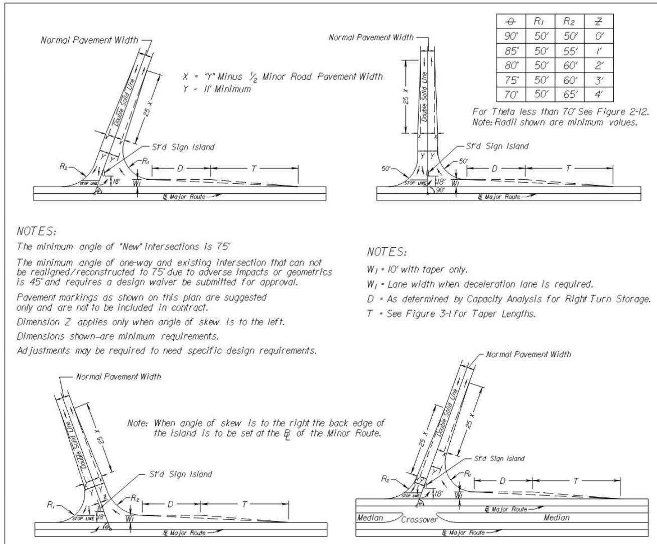
**FIGURE 2-11 INTERSECTION DESIGN FOR RURAL APPLICATIONS WITH OR WITHOUT STANDARD SI-1 SIGN ISLAND DESIGN\***
