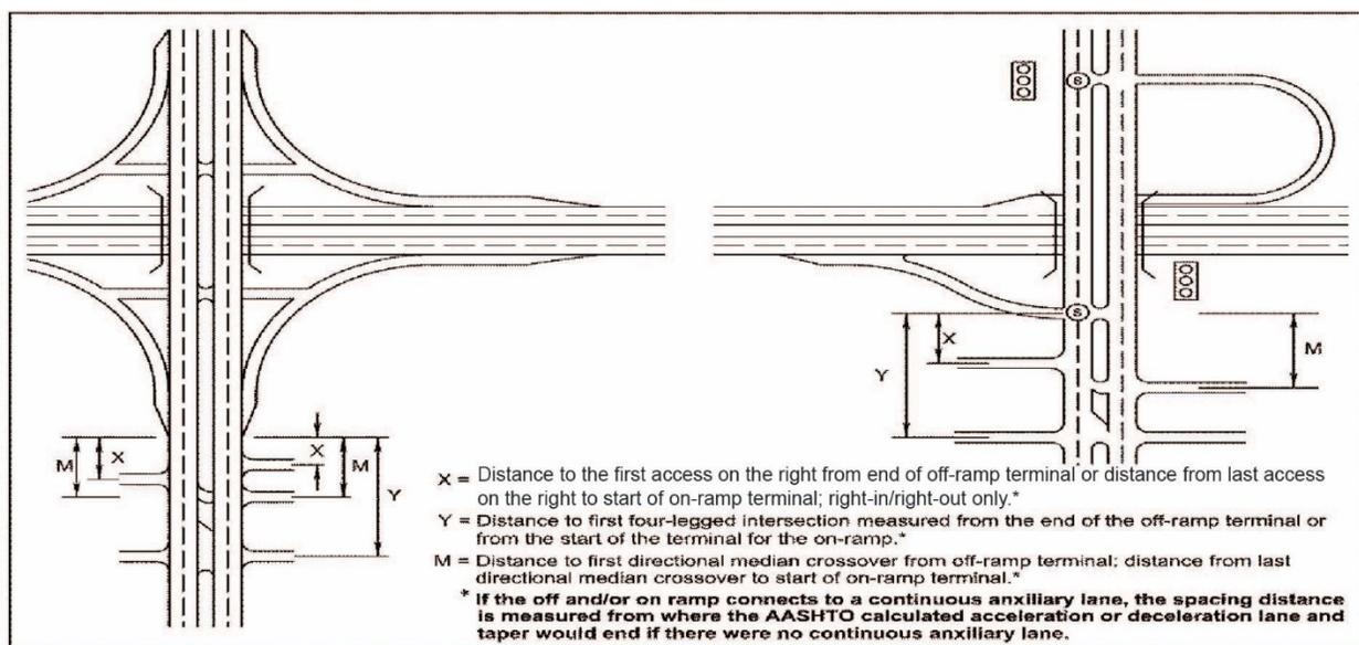
**FIGURE 2-9 ACCESS CONTROL ON MULTILANE CROSSROADS AT INTERCHANGES**
