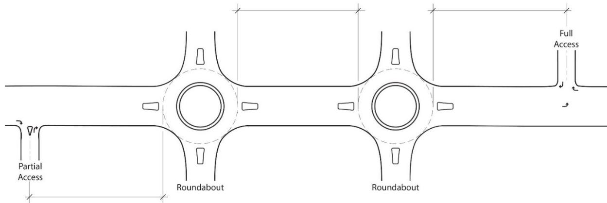
When determining the distance between a roundabout and another access, the measurement is not taken from the centerline. Instead, the point of reference is the outer edge of the inscribed circle diameter (Yield Line) on the nearest approach.
