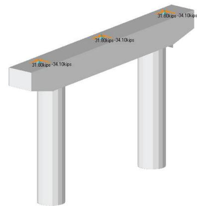
Figure 4.3.2(2): Design of the Piers Using RCPier Software
