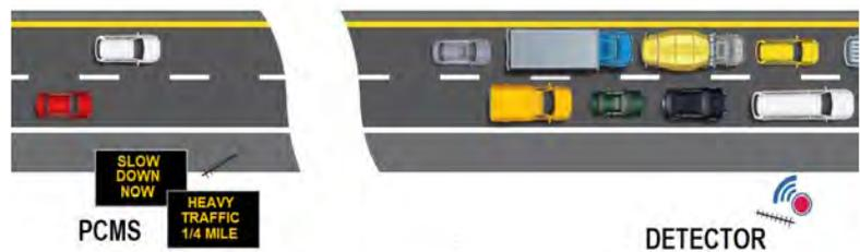
Figure 4.5.2.9 - Queue Detection and Warning System
