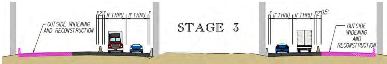
Figure 4.5.3.2.10 - Stage 3 Traffic Condition at Exit 205
