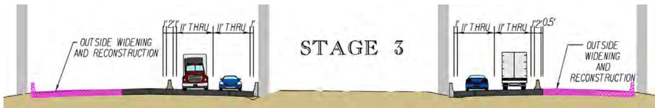
Figure 4.5.1.10 - Stage 3 Traffic Condition at Exit 205
