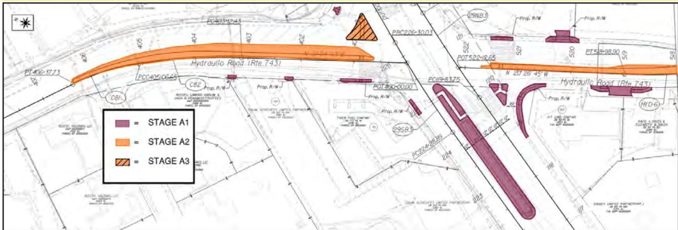
Figure 4.5.1.1: Construction Stages - Element A
