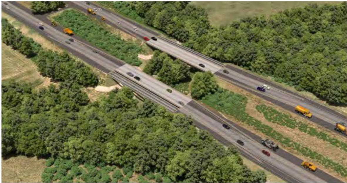
Roadway remains shifted to the right; traffic on bridges is shifted to the left; traffic shifts are required between roadway and bridges
