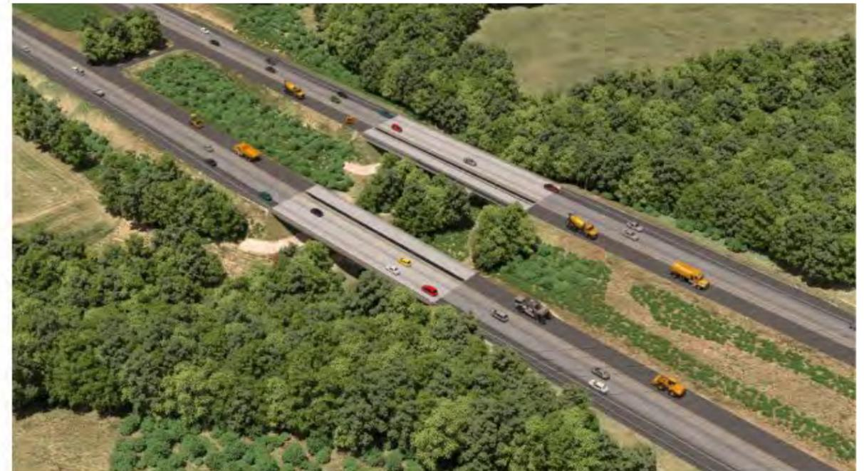
Roadway and bridges are two lanes but are shifted to the right; traffic shifts are required between roadway and bridges
