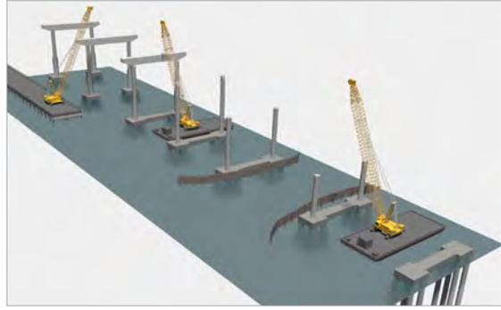
**Figure 4.5-3: HRB Sequence Step 2.** Construct bridge footings, columns, and caps on land and water piers concurrently. Each of the three areas – east bank, river, and west bank – will typically have dedicated equipment resources, but share labor resources. A unique feature of the marine “waterline footings” is that GPC will use precast stay-in-place forms to facilitate construction.
