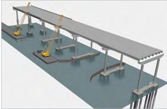
**Figure 4.5-5: HRB Sequence Step 4. Deck and parapet concrete placement.** The HRB deck and parapets will be cast-in-place. The deck concrete will typically be pumped and the parapet will be placed directly from redi-mix trucks. All work over the navigable channel, Bainbridge Blvd, Libertyville Blvd, and the rail lines will require coordination to protect the traveling public, but the emphasis will be on shielding and other precautions to isolate the construction work.
