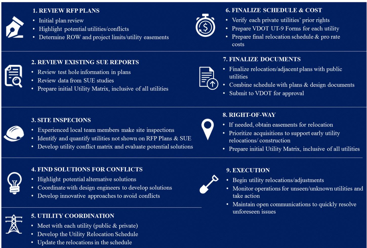
Figure 4.4.2-1: Flowchart for addressing utilities on the Project
