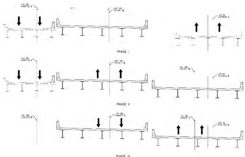
**Conceptual bridge staging to eliminate phasing of SBL construction.**
