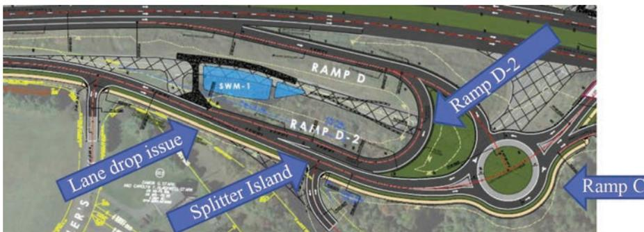
**Impact:** The RFQ design of eastern roundabout may not be feasible for requested design vehicles or for maximizing safety.
