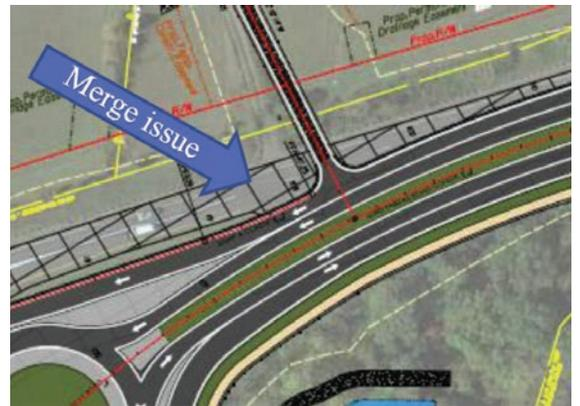
**Mitigation:** Using the ATC process and an operational analysis, we will investigate eliminating the bypass lane or reconfiguring the area such that vehicles in and around the western and southern legs of the roundabout will maintain closer to equal speeds, thus increasing safety.
