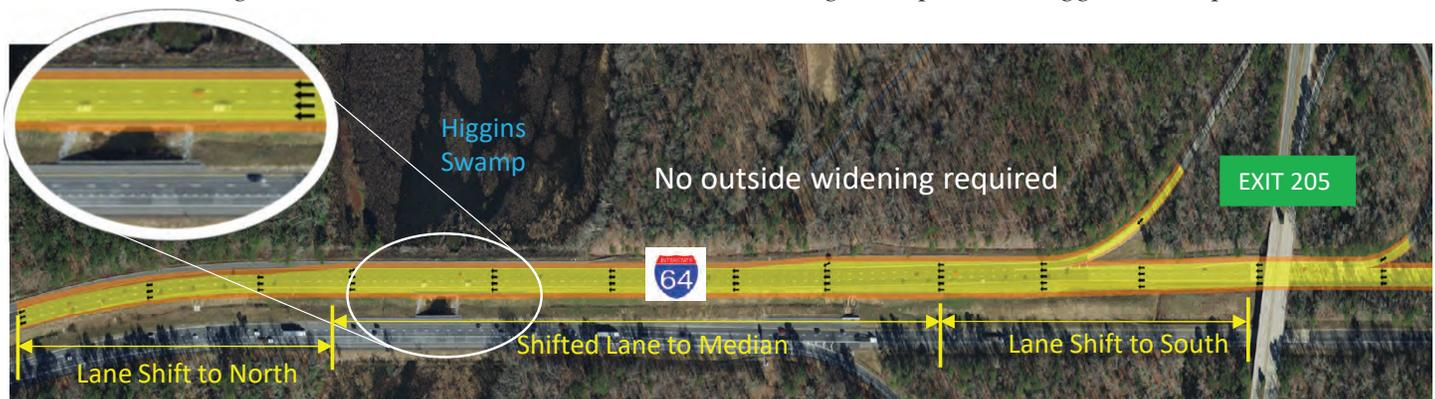
Another alternative involves separating the two entrance ramps onto WB I-64 providing back to back acceleration lanes, tapers, and separation meeting AASHTO standards. Increasing the entrance curve radii to 35 mph of the NB to WB on-ramp will reduce the required acceleration lane and potentially allow all improvements to end prior to the box culvert at Sta 4998. Any potential geometric solution will be evaluated to ensure proper traffic and safety operations and minimize environmental impacts.
