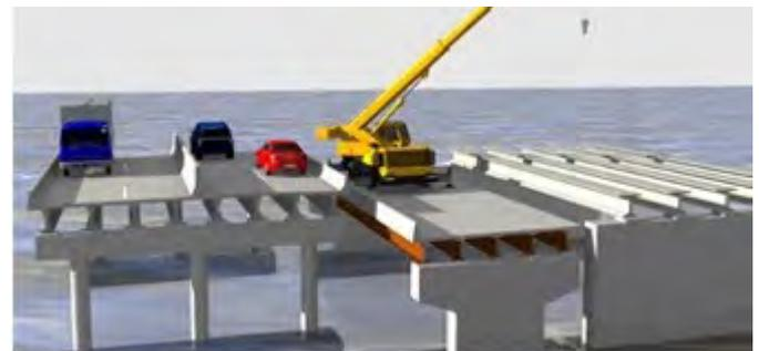
**Figure 4. EB Bridge reconstruction utilizing staged top down construction eliminating the temporary work bridge between the WB & EB.**
