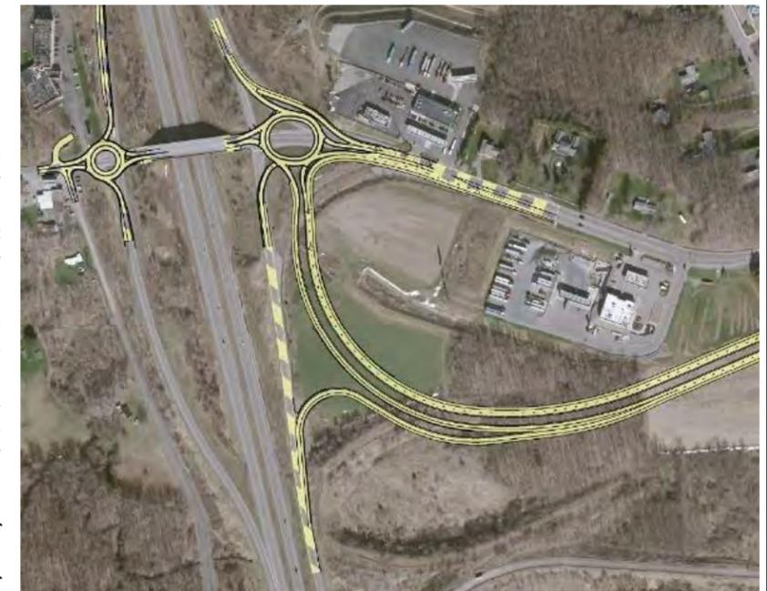
**AMT's Roundabout Interchange Configuration (Selected for Design)**
