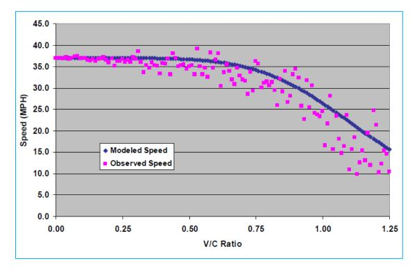
Figure 10.3 Example Comparison Plot of Speeds versus Volume/Capacity Ratios
