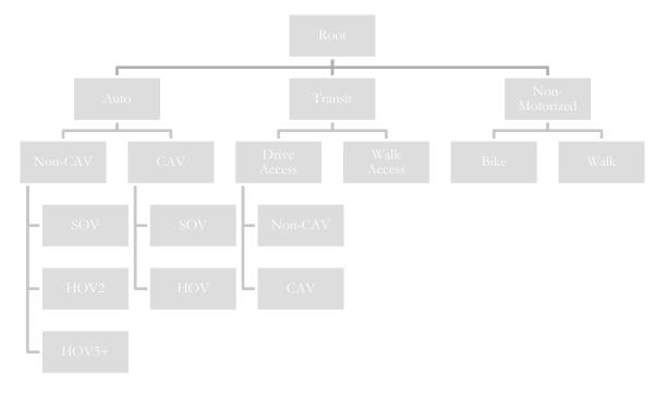
Figure 2.5 An Example of Mode Choice Structure with CAVs
