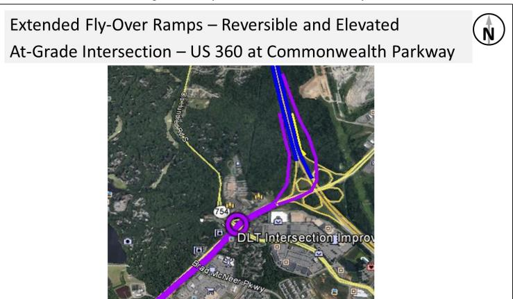
Figure 23: Concept #29 – Grade-Separated Intersection
