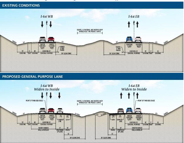
Figure 2-2. Existing and Build Condition Typical Sections
